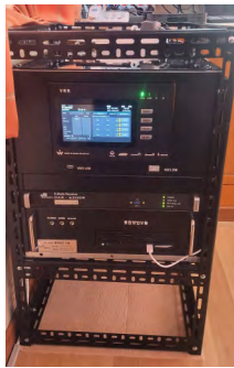
Fig. 4. Ship-mounted VDES R-Mode receiver and reception server.
