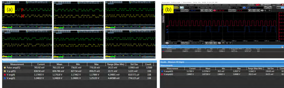
Fig. 13. Detailed image of verification result: (a) LVDS (signal 4~6) and (b) LVTTTL signals (SPI interface).
