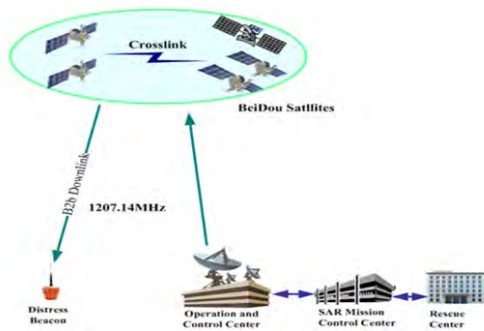
Fig. 8. Concept of BDS SAR return link service (Yang et al. 2019).
