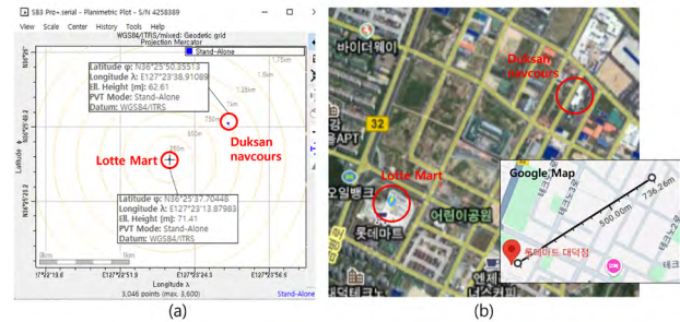
Fig. 10. Static scenario: position manipulation commands and target receiver position result (a) planimetric plot from Septentrio application (b) spoofing position setting in spoofing control application.
