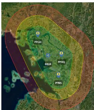
**Fig. 3.** VBS-PPK coverage map for four base stations of PPHS, IHUB, PPGH, and PPHQ.
